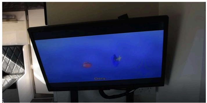
As part of the options pack you are provided with a 19inch HD TV. To operate the TV you need to power up the TV via the control panel (for hybrids) or by connecting the TV to an available CIGA connection and ensuring that the Sockets button on the control panel is on.
