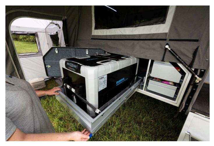
By pressing the blue latch at the front of the slide in the downwards position, this will release the fridge slide lock and allow the fridge to slide in and out of its storage compartment. The fridge storage section includes both a Ciga and Anderson plug providing you with 2 options to power your fridge. To power your fridge, you must turn the fridge power switch to the on position on your control panel.
