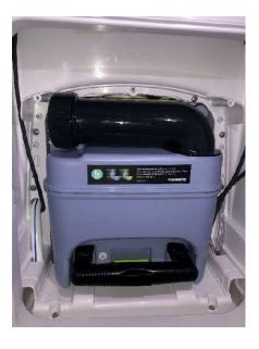
To remove the cassette, lift the green tab behind the pull out black handle as see below:
