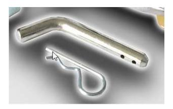
11. Once the coupling/hitch is locked in place, ensure the positive locking pin is locked in. Next fully raise the jockey wheel before unclamping it and rotating the jockey wheel, finally, locking it fully raised
