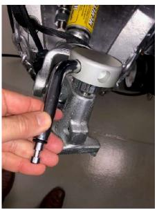
The images above show how to release the safety switch and unwind the hitch cap with the locking pin at the same time.
