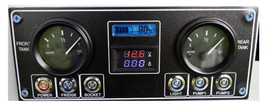
As the image above shows the charge of the batteries is 80% and the actual voltage of the batteries is 12.6V. The trailer is not drawing any amps from the battery. As you start to turn on the internal lights, the fridge or the pumps the amperage will increase. This indicates that the batteries are being used. You should charge your batteries to full charge prior to travelling
